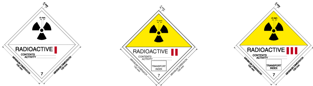
Figure 1. Transport labels – reproduced from Figures 2, 3 and 4 of the IAEA Regulations
